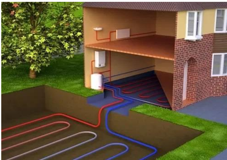
Figure 4 - example of a GSHP trench-loop circuit
